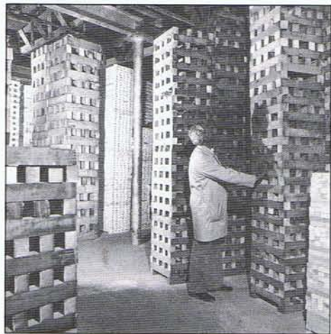
Modern techniques are used to scientifically cure the quarter-sawn cantlins.
