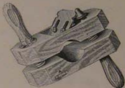
3364 Best Beech Fork Shaft Rounders, with Beechwood Screws, adjustable down to 1 1/2 in. dia. 24/- each
